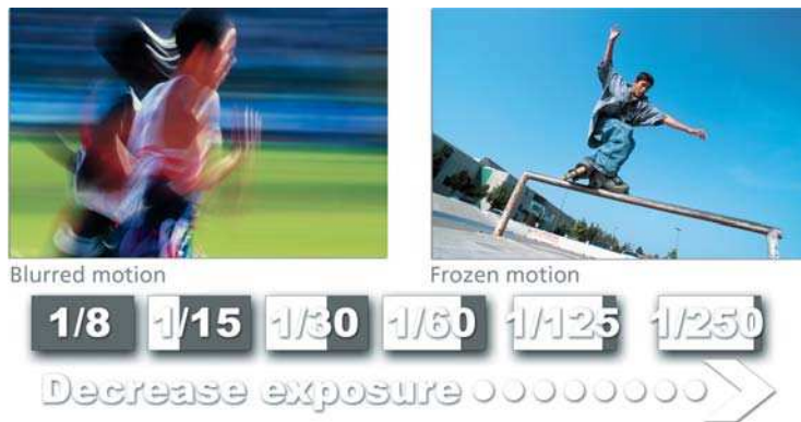
Figure 8.3 The shutter speed controls both the amount of light entering the camera and the way that action or movement is captured. Fast shutter speeds freeze the action, whereas slower settings blur the movement.
